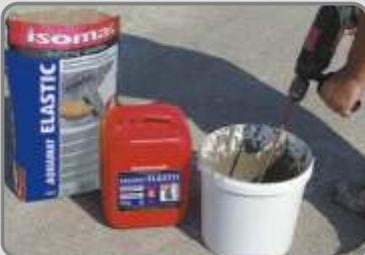
The content of component A (mortar) is added into the liquid component B (elastifying agent) and the indicated water, under continuous stirring, until a uniform viscous mixture of **AQUAMAT-ELASTIC** is formed.
